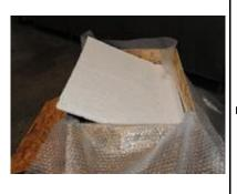
Novel class of insulating panels based on nanomaterials derived from renewable resources to be used for building energy efficient retrofitting. Panels are suitable for three fully operational components: internal and external insulation as well as internal partition.
